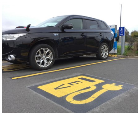
EVs with bi-directional charging capability will be able to power up from solar and also put power back into the home or business when needed
